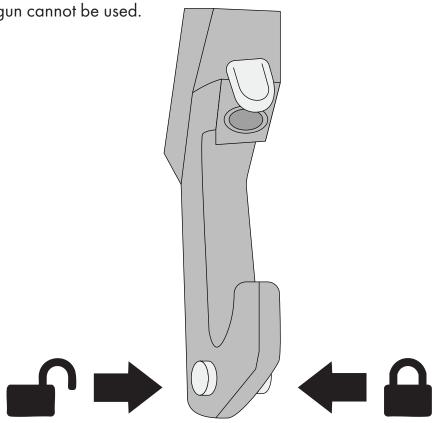
After turning off the lock, use the trigger to spray the water. ALWAYS point the gun at the ground first.
