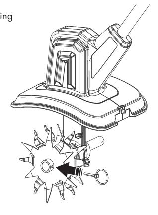
Put the ring of the locking pin around the axle.
