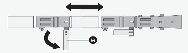
Unclip the telescoping lock (M) to release the pole. Extend the pole to the desired length.
