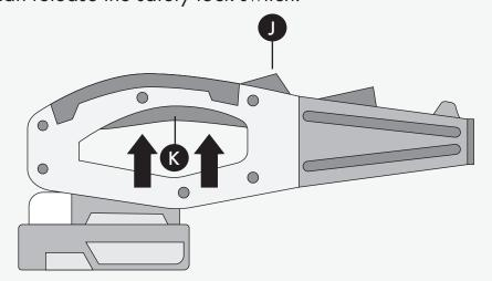
To turn the tool OFF, release the trigger switch (K)
