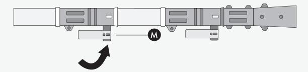
Lock the pole in position by closing the telescoping lock (M), ensuring the pole is secured.
