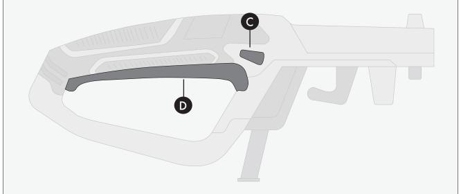
To turn the tool OFF, release the trigger switch (D)
