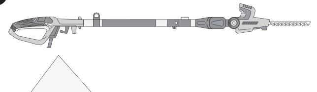
To turn the hedge trimmer ON, push and hold the safety lock switch (C) located on the handle forward with your thumb, then squeeze the trigger switch (D) with your fingers. Once the tool is running, you can release the safety lock switch.
