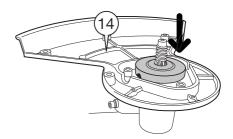
Place the Brush Cutter Disc (16) over the drive shaft so it sits flush on top of the Coupling Plate (20).
