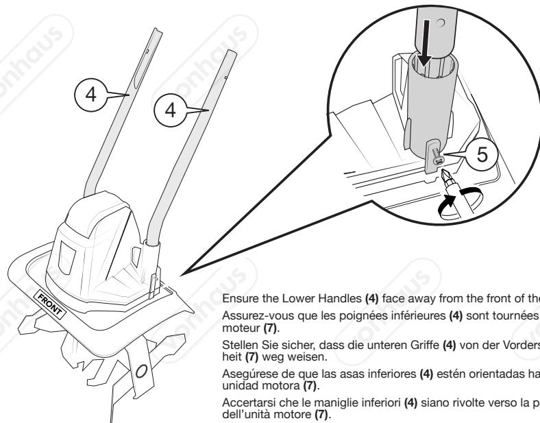
Ensure the Lower Handles (4) face away from the front of the Motor Unit (7).
