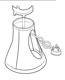
Place the power cord into the center hole of the Front and Rear base, and then assemble the Front Base to the Rear Base.
