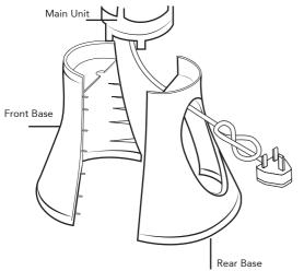
Place the power cord into the center hole of the Front and Rear base, and then assemble the Front Base to the Rear Base.
