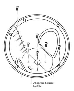
Align the Square Hole up to the Square notch on the Main Unit, and insert the screws.
