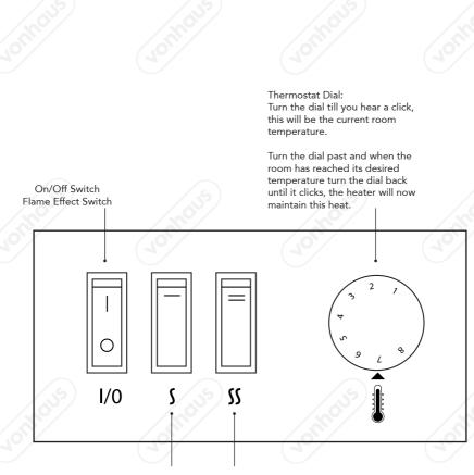
I Switch: Press this to activate low heating (950W).
