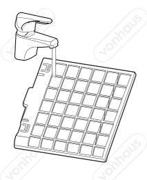
Clean debris from the filter using a soft bristle brush then with clean running water do not use any detergents or abrasive chemicals, rinse the filter thoroughly and leave to completely dry for 24 hours
