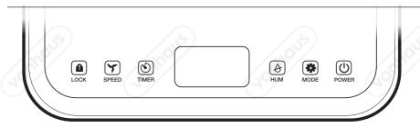
**POWER:** : When the unit is powered on the indicators and LED will display for 1 second after a "buzz" is heard the power indicator will be in standby mode.
