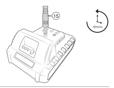
Plug the Battery Charger (15) into a suitable mains power outlet. Insert the opposite end into the top of the Battery to begin charging.
