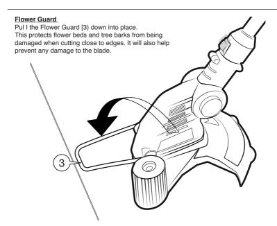
The Flower Guard can also be used to prevent blades encountering any material denser than grass. Such as lawn edging, paving, fencing or stone/wood borders.
