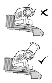
Ensure the edges of the Blade Holder and Safety Guard (circled) align before use. If they are not aligned, then the Saftey Guard has not been fitted correctly.
