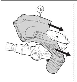
Push the Safety Guard under the Blade Holder until it 'clicks' into position.
