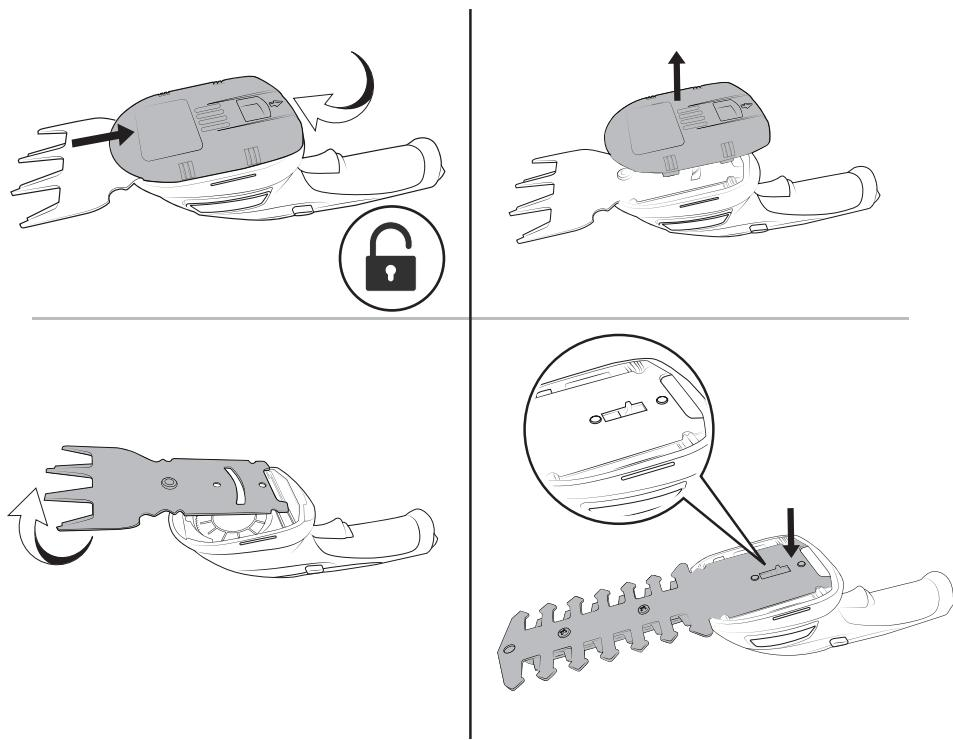
If you are having difficulty attaching the Hedge Trimmer Blade to the Main Unit, the gear cam may not have aligned with the white moulding on the blade. Position the Blade as shown and apply some pressure with one hand. Using the other hand, gently press the Power Trigger until the gear aligns.
