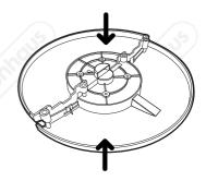
**2.** Invert the Main Unit (**3**) and align the assembled base with the 4 screw holes on the bottom of the Main Unit. Use the 4 Fixing Screws (**6**) supplied to attach the two together.
