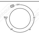
**NOTE:** Both the Timer and Speed control must be on for the product to operate.
